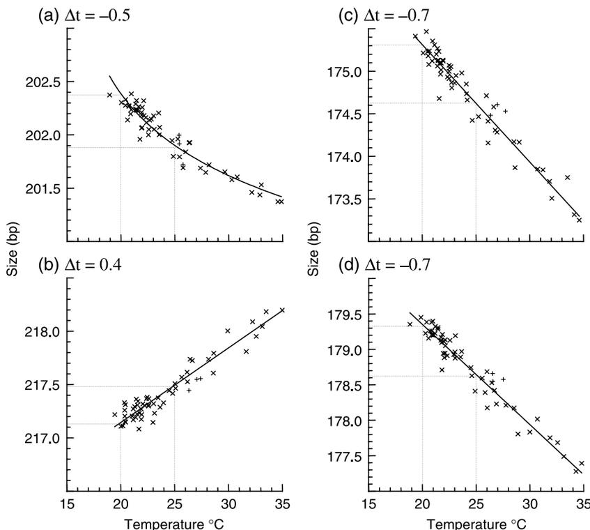
**Fig. 1** Correlation of internal (block) machine temperature with estimated allele size for two microsatellite loci. Laboratory temperature is 1–2 °C lower than internal temperature. The points marked by a + are the estimated sizes, using chilled buffer, plotted against internal temperature. (a) *Mpo9* allele 1 and (b) 2. (c) *Mpo11* allele 1 and (d) 2. For both alleles of *Mpo8*, the relationship was similar to (a), whereas for *Mpo10* it was like (c) and (d).
